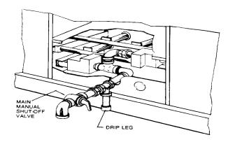
FIGURE 6 - EXTERNAL SUPPLY CONNECTION EXTERNAL SHUT-OFF
